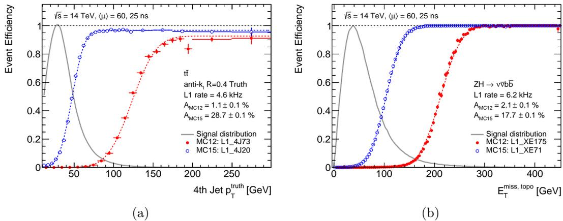
Figure 7.5: Level 1 event efficiency turn-on curves for (a) four-jet triggers in  $t\bar{t}$  events and (b)  $E_T^{\text{miss}}$  triggers in  $ZH \rightarrow \nu v b \bar{b}$  events. The trigger thresholds indicated in the legends have been selected for the same trigger rate in the MC12 and MC15 simulations.
