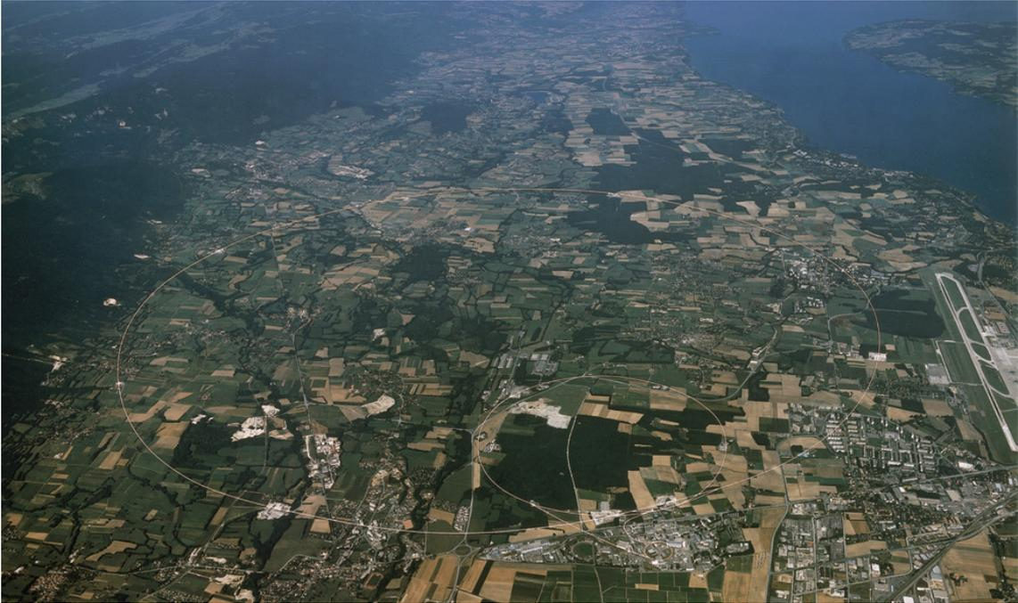
Figure 3.1: Aerial view photograph of CERN with the paths of the accelerator rings superimposed. ©CERN.
