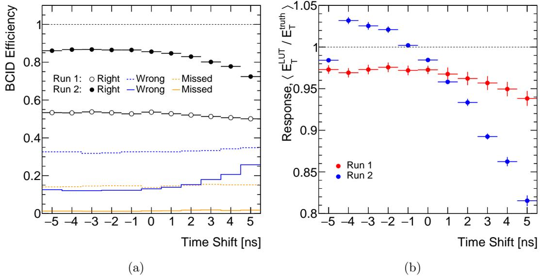
Figure 6.15: FCal1 performance comparison in the TOYMC between the Run 1 and Run 2 configurations for systematic timing shifts from  $-5$  ns to  $+5$  ns. Subfigure (a) shows the BCID efficiency for 5 GeV signals. The black points show correctly identified signals, the blue lines show where the peak-finder fires one bunch crossing early or late, and the yellow lines show the signals missed by the peak-finder. Subfigure (b) shows the response for 30 GeV signals.
