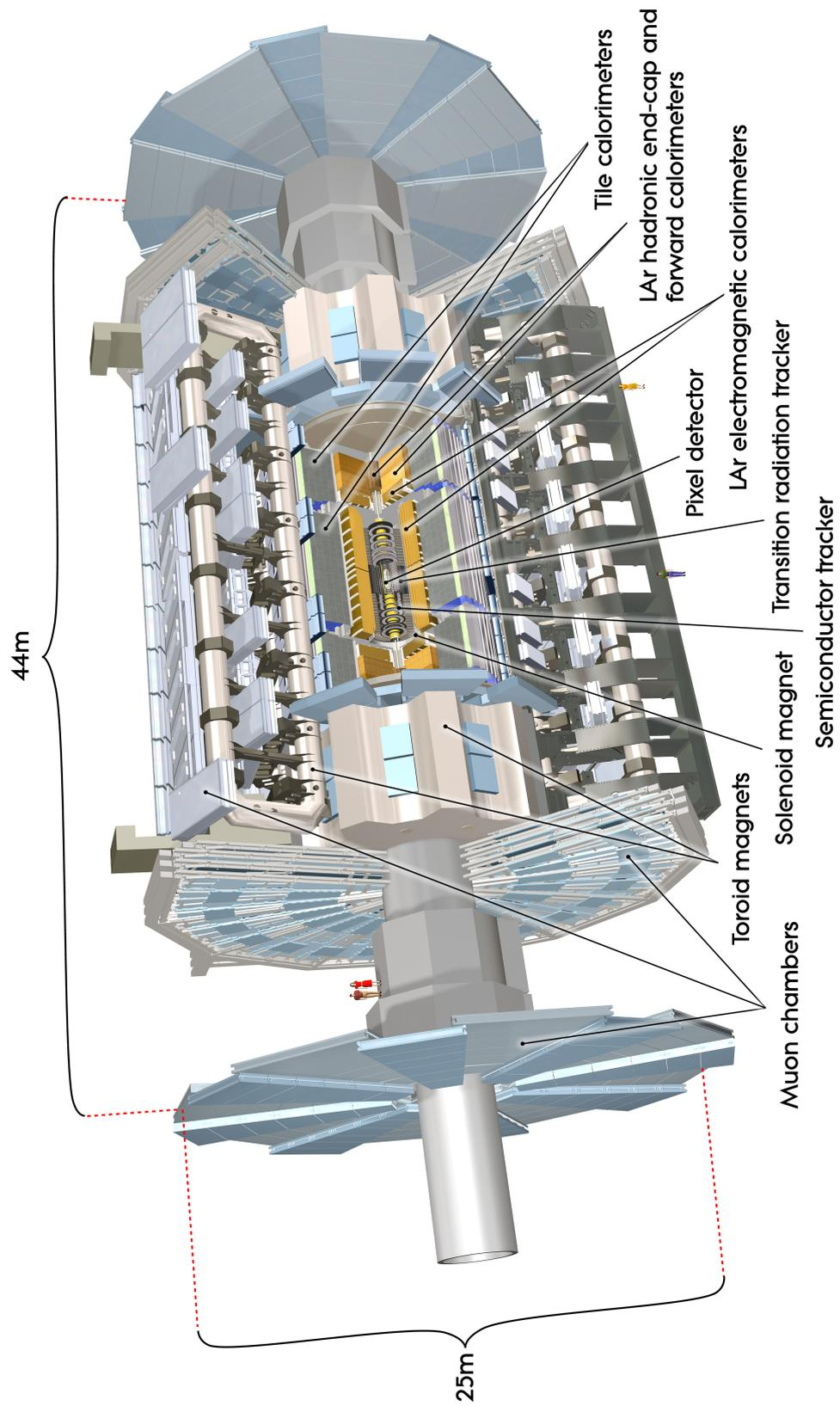
Figure 4.1: Cut-away view of the ATLAS detector. ©CERN.
