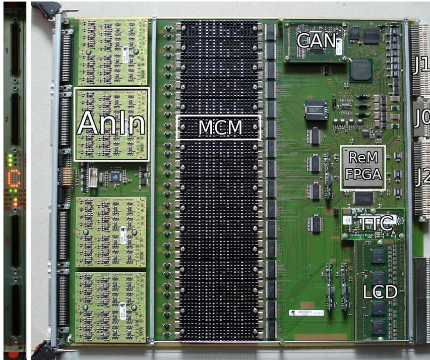
Figure 5.2: Photograph of the PPM front panel (left) and the board top view (right). The analogue signals enter the module on the left-hand side and are managed by four AnIn boards. At the centre are sixteen MCMs which digitise the signals and perform the BCID algorithms programmed into an on-board ASIC. The right-hand side of the board contains one LCD, one TTC Decoder, one CAN module, and a ReM FPGA. Taken from [94].
