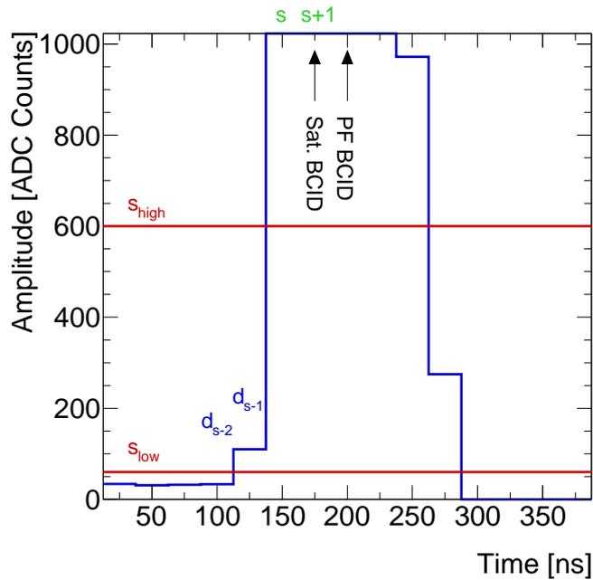
Figure 5.5: Illustration of the BCID algorithm for saturated signals. The two ADC values  $d_{s-2}$  and  $d_{s-1}$  are compared to the programmable thresholds  $s_{low}$  and  $s_{high}$  to determine if the correct bunch crossing is  $s$  or  $s + 1$ . In this case, the peak-finder BCID fires one bunch crossing late.
