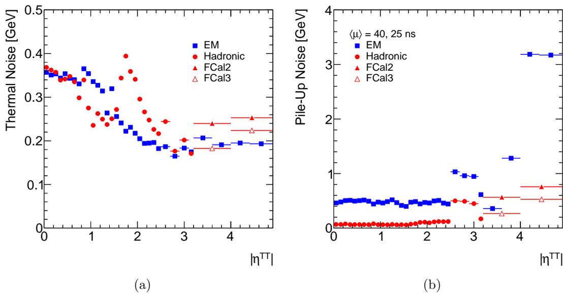
Figure 6.1: Calorimeter noise as transverse energy determined by the standard deviation of ADC distributions as a function of the trigger tower  $|\eta|$  for (a) thermal noise and (b) pile-up noise. See Sections 6.2.1 and 6.2.2 for more detail.
