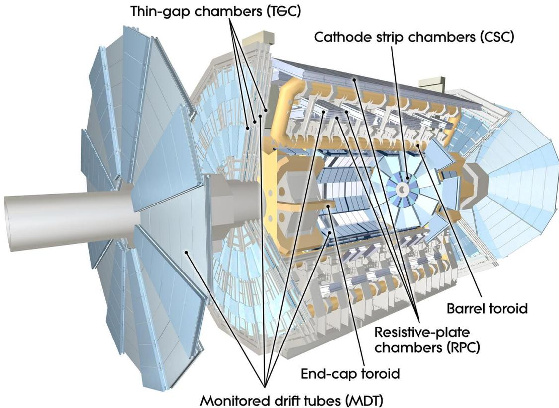
Figure 4.5: Overview of the ATLAS muon systems. ©CERN.
