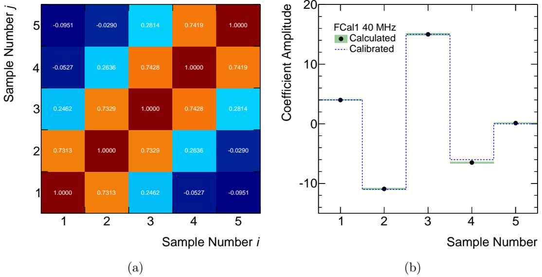
Figure 6.7: Calibration of filter coefficients for a trigger tower in FCal1 with 40 MHz sampling and 25 ns bunch spacing. (a) shows the correlation matrix  $\mathbf{R}$  between samples and (b) shows the corresponding filter coefficients  $\mathbf{a}$  after normalisation.
