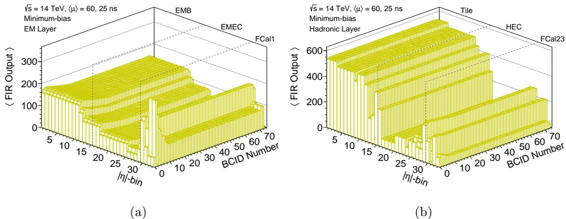
Figure 7.2: Average FIR output of the autocorrelation filters in minimum-bias simulated events per  $|\eta|$ -bin and over one bunch train for trigger towers in (a) the EM and (b) hadronic calorimeter layers.
