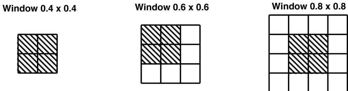
Figure 5.7: Jet trigger algorithm operates on jet elements indicated by the  $0.2 \times 0.2$  grid. The three available  $E_T$  cluster sizes of  $2 \times 2$ ,  $3 \times 3$  and  $4 \times 4$  jet elements are shown with the corresponding RoIs given by the shaded regions. Taken from [76].
