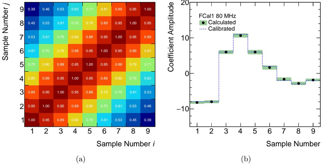
Figure 6.9: Calibration of filter coefficients for a trigger tower in the EMEC IW with 80 MHz sampling and 25 ns bunch spacing. (a) shows the correlation matrix  $\mathbf{R}$  between samples and (b) shows the corresponding filter coefficients  $\mathbf{a}$  after normalisation.
