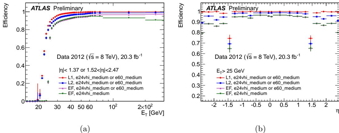
Figure 4.7: Single electron trigger efficiencies after the L1, L2 and EF selections as a function of (a) the offline electron  $E_T$  for pseudorapidity ranges of  $|\eta| < 1.37$  or  $1.52 < |\eta| < 2.37$  and (b) the offline electron  $\eta$  for  $E_T > 25$  GeV. The efficiencies were measured with a tag-and-probe method using  $Z \rightarrow ee$  decays for the `e24vhi_medium1` OR `e60_medium1` trigger and are shown with combined statistical and systematic uncertainties [91].
