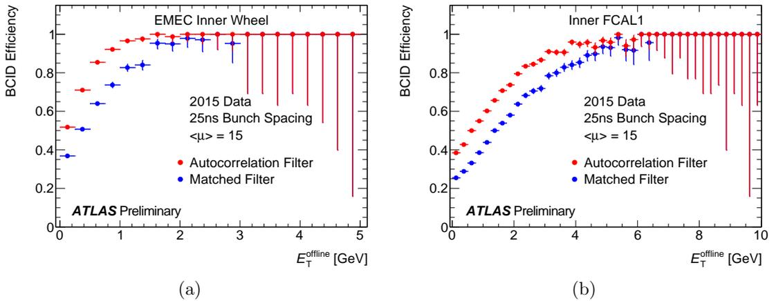
Figure 7.19: The efficiency that a calorimeter pulse is identified in the correct bunch crossing as a function of the offline  $E_T$  [124]. The performance of the matched filter is compared to the autocorrelation filter for (a) the EMEC IW and (b) FCal1.
