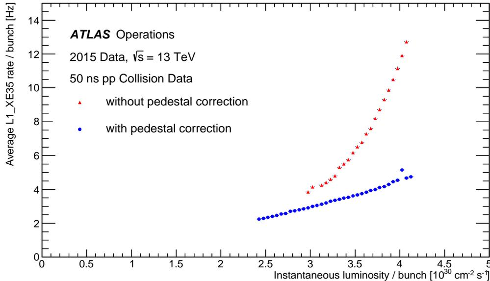
Figure 7.20: Level 1 trigger rate per bunch as a function of the instantaneous luminosity per bunch for the  $E_T^{\text{miss}}$  trigger with a 35 GeV threshold [124]. The rates are shown with and without the pedestal correction applied.
