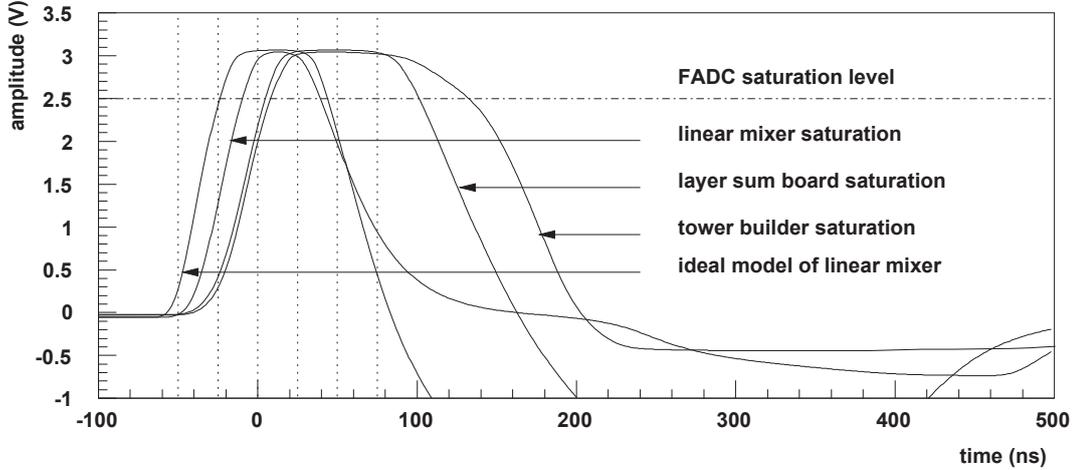
Figure 5.4: Pulse shapes for saturated trigger tower signals at different stages of the LAr summing chain. Taken from [96].
