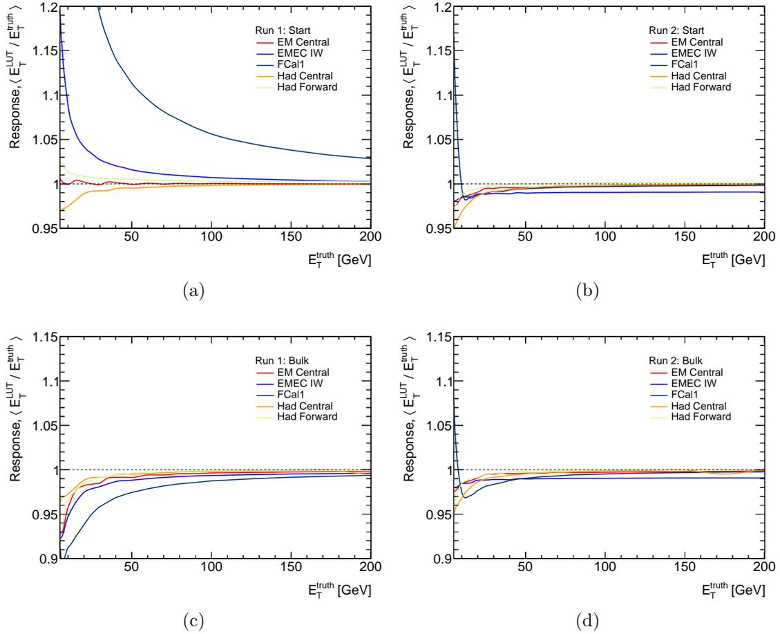
Figure 6.13: Trigger tower  $E_T$  response in the TOYMC as a function of the signal pulse  $E_T$  in different calorimeter regions. Subfigures (a) and (b) are for the Run 1 and Run 2 configurations at the start of the bunch train. Subfigures (c) and (d) are for the Run 1 and Run 2 configurations in the bulk of the bunch train.
