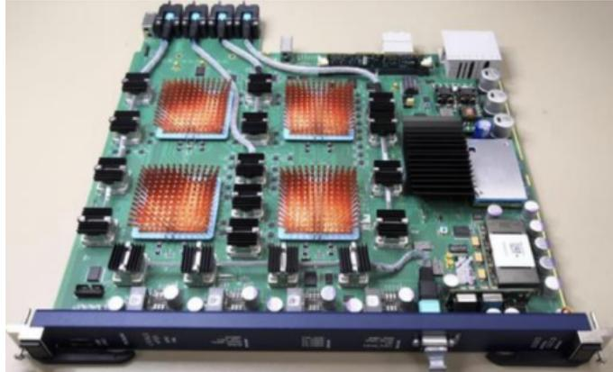
Figure 4.3: A photo of the eFEX module. There are four processor FPGAs under the copper heatsinks. Photo taken from Ref. [106].
