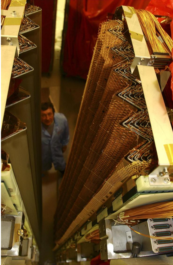
Figure 2.12: Electromagnetic calorimeter barrel section showing its accordion shape. [11].
