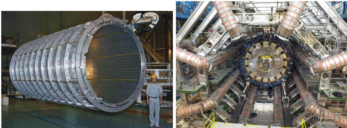
Figure 3.8: An illustration of the barrel solenoid (left) and toroids (right) used at ATLAS [34].
