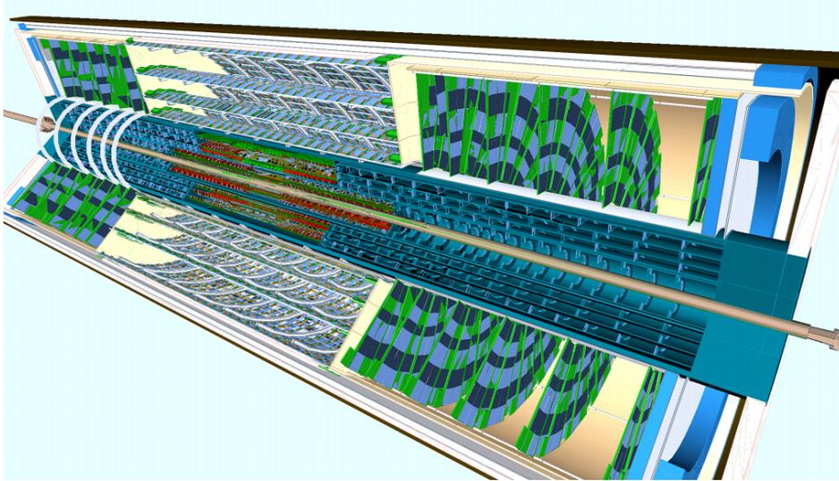
Figure 4.1: Diagram of the ATLAS ITk as implemented in the GEANT4 simulation programme [71]. The beampipe is shown in brown at the centre of the diagram; surrounding this are the pixel and strip detectors which both extend the full length of the diagram.
