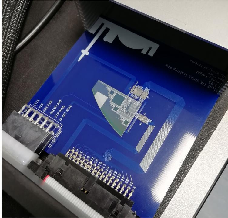
Figure 4.5: ITk QA test chip setup: silicon QA piece mounted on a PCB which is secured inside the testing box.
