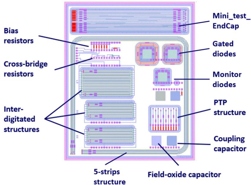
Figure 4.4: Diagram showing structures on the test chip taken from [78]. Labels added.
