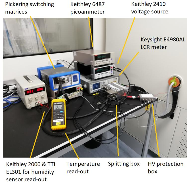
Figure 4.6: ITk QA test chip setup: measurement instruments and splitting matrices, along with splitting box and high voltage (HV) protection box shown next to the climate chamber.
