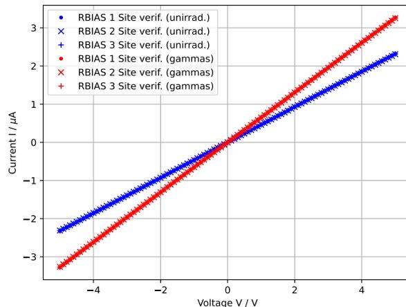
Figure 4.10: Plot of IV scans of bias resistors on the site verification test chips (one unirradiated, one gamma irradiated). IV curves are shown in blue for unirradiated devices and red for gamma-irradiated devices. For each device, three IV curves are shown corresponding to each resistor which can be tested with wire-bonds.
