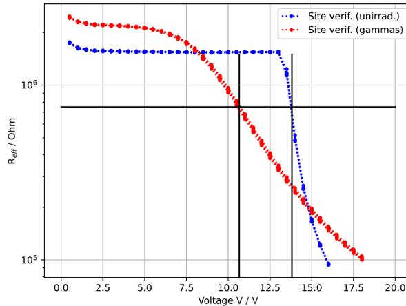
Figure 4.11: Plot of effective resistance from IV scans of PTP structures on the site verification test chips. Curves corresponding to the five PTP structures which can be probed are shown for each device. Curves are shown in blue for unirradiated devices and red for gamma-irradiated devices. The horizontal black line corresponds to a resistance of  $0.75 \text{ M}\Omega$ , corresponding to half the nominal  $R_{\text{bias}}$ .
