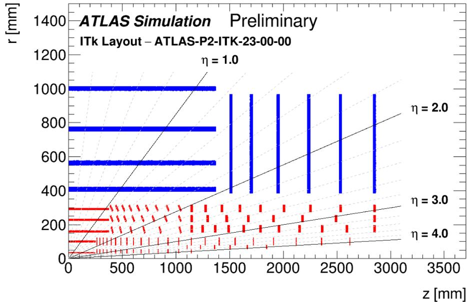
Figure 4.3: Layout of the ATLAS Inner Tracker upgrade (ITk) [77]. Layers of the pixel and strip detector are shown in red and blue, respectively.
