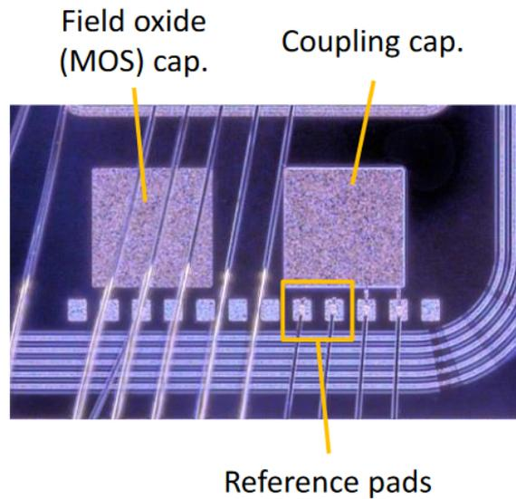
Figure 4.7: Image of test chip showing coupling capacitor and field oxide capacitor structures with spare wire-bonding (“reference”) pads labelled.
