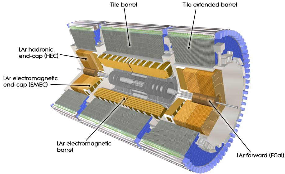
Figure 3.5: Diagram of the ATLAS calorimeters [66].
