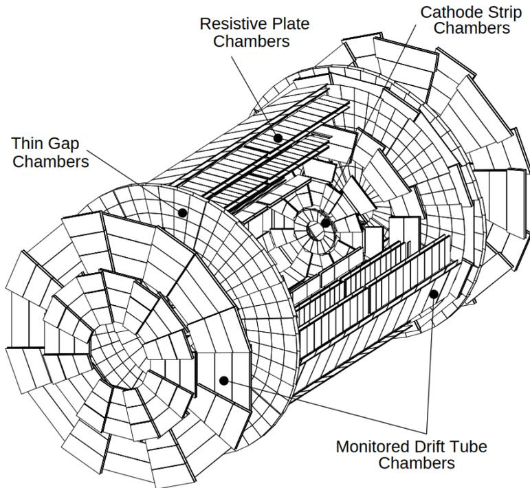
Figure 3.6: Diagram of the ATLAS muon spectrometer [68].
