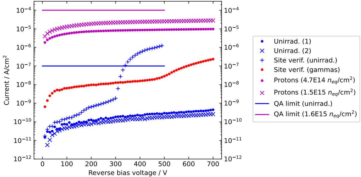
Figure 4.8: Plot of MD8 current between pad and backplane as a function of bias voltage for six MD8 devices. IV curves are shown in blue for unirradiated devices, red for gamma-irradiated devices, and magenta for proton-irradiated devices. Currents for the unirradiated devices have been corrected to  $-20\text{C}$  using Eq. (4.3). Also shown are the maximum current limits permitted by the ITk QA requirements up to 500 V.
