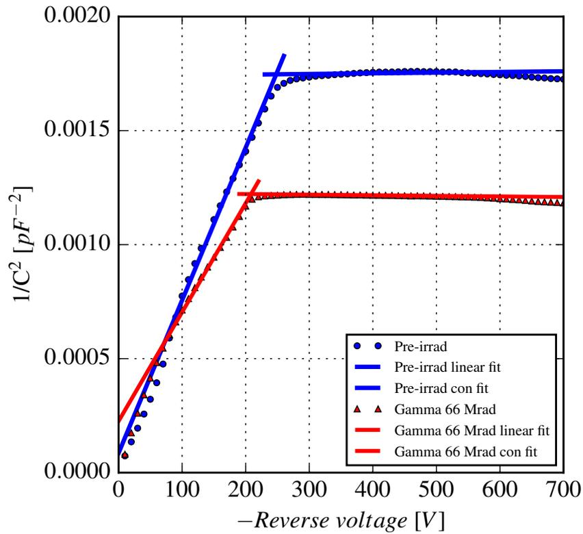
Figure 4.9: Plot of MD8 bulk capacitance as a function of reverse bias voltage for two MD8 devices showing the extraction of the full depletion voltage. Plot produced by Dr Ioannis Kopsalis. Measurement data are shown as markers while solid lines represent linear fits to the rising slope (“linear”) and constant plateau (“con”).
