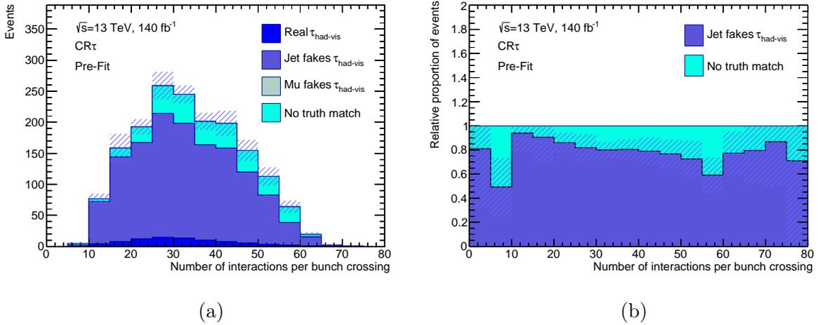
Figure 6.9: Distribution of (a) number of interaction vertices in each event and (b) relative fraction of unknown objects faking  $\tau_{\text{had-vis}}$  as a function of this variable in  $\text{CR}\tau$ . Events are classified according to whether the  $\tau_{\text{had-vis}}$  is truth-matched to a real  $\tau$  lepton, a jet, a muon, or is not truth matched. The hatched band represents the MC statistical uncertainty.
