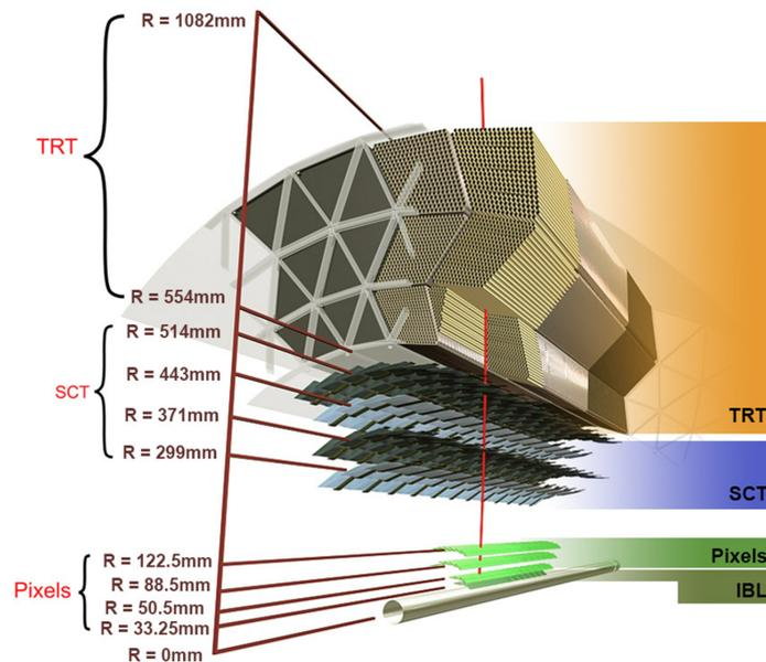
Figure 3.4: Diagram of the ATLAS inner detector [64].
