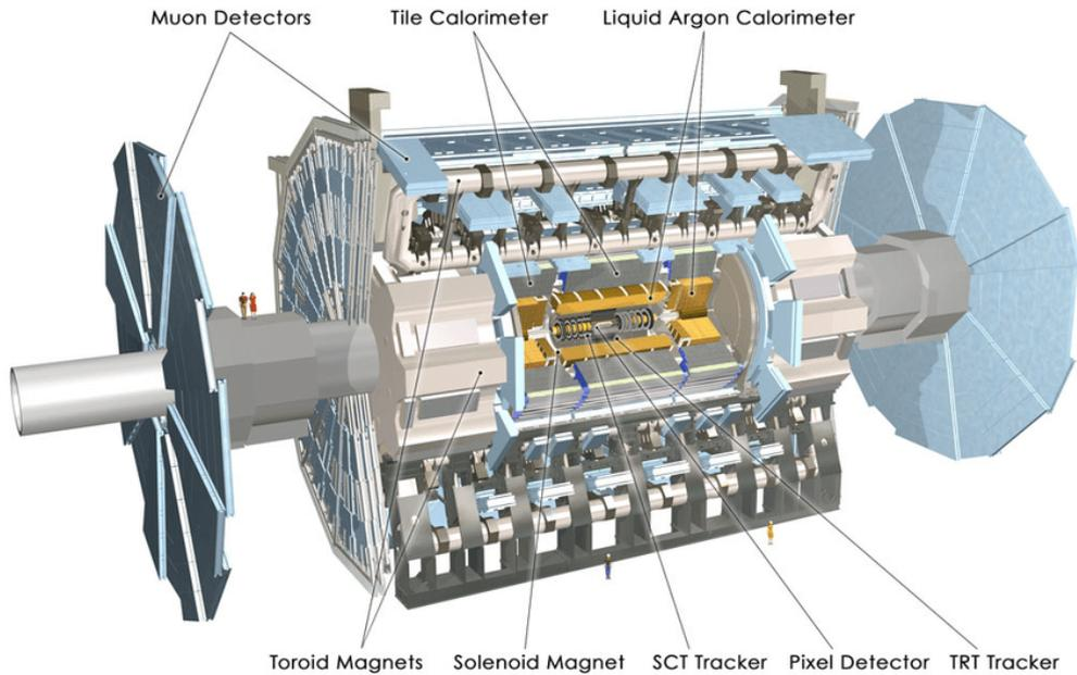
Figure 3.3: Diagram of the ATLAS detector [63].
